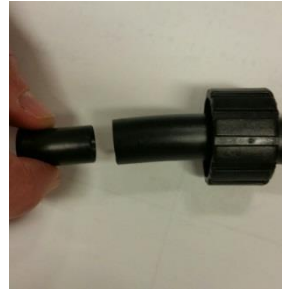
Install "insert" inside tubing.
