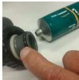
2. Lubricate ALL BLACK ORINGS with Silicone lubricant.
