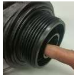
2. Lubricate ALL BLACK ORINGS with Silicone lubricant.
