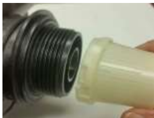
3. Install upper basket (insert and twist to lock in place).
